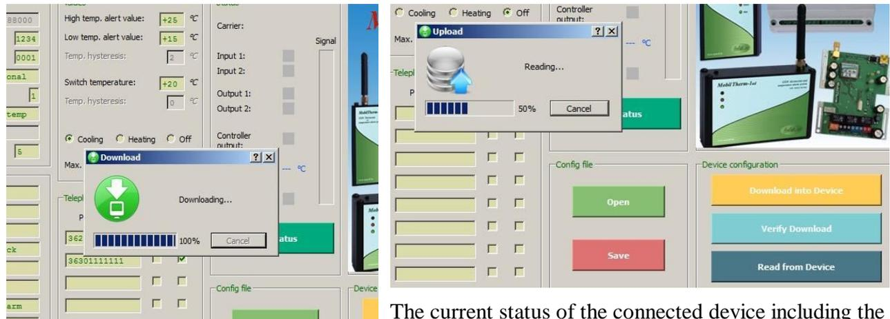
The current status of the connected device including the inputs, the outputs, the control outputs, the current temperature, the power voltage, the current network coverage of the provider and the industrial GSM modem can be displayed by using the status update button.
