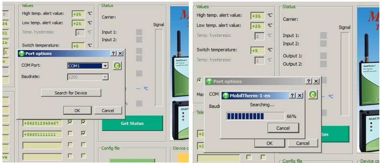
software will automatically search and recognize the connected device. After successful recognition, the corresponding picture of the device will be displayed in the main window of the software. The status of the device can be queried by pressing the **Get Status** button if the device is connected to a network. After connecting the device and querying its status, the screen is represented as follows:
