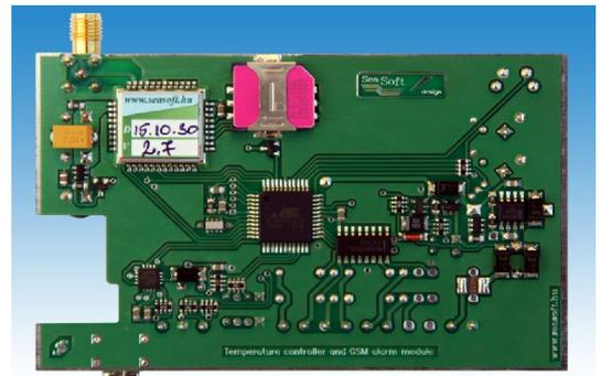
resettable fuse also has been installed into the device. It can be configured via its **mini-USB** port at the bottom, and the configuration settings can be downloaded, loaded
