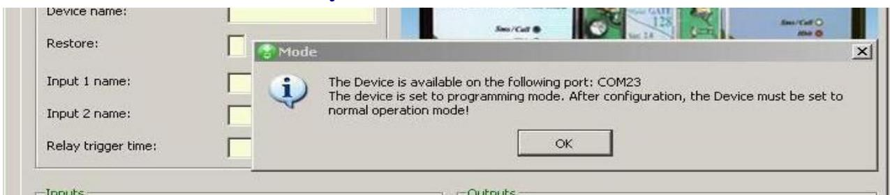
The GSM device has to be identified by which serial port from **Com1...Com99** it is connected to.
