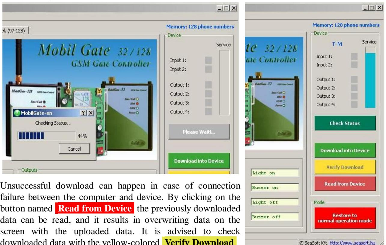
Unsuccessful download can happen in case of connection failure between the computer and device. By clicking on the button named **Read from Device** the previously downloaded data can be read, and it results in overwriting data on the screen with the uploaded data. It is advised to check downloaded data with the yellow-colored **Verify Download**
