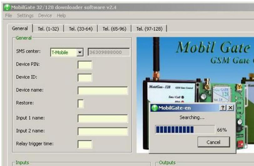
module driver the serial port configuration. It starts by clicking the **Set Port** button. Windows registers the device and assigns it to a COM-xx port. The software indicates module version and enters configuration mode. The user can configure *MobilGate-128* controller freely in configuration mode. If the software cannot find the port of the device indicated on the picture, it has to be identified manually in Windows by the followings:
