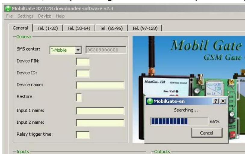
Windows registers the module and assigns it to its **COM port**. The downloader indicates module classification by activating its coloured controls and **enters configuration mode**. The user can configure MobilGate GSM gate opener freely in configuration mode.
