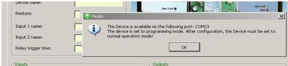
You have to find the device indicating which serial port it is connected to, from **Com1 to Com99**, by your computer.
