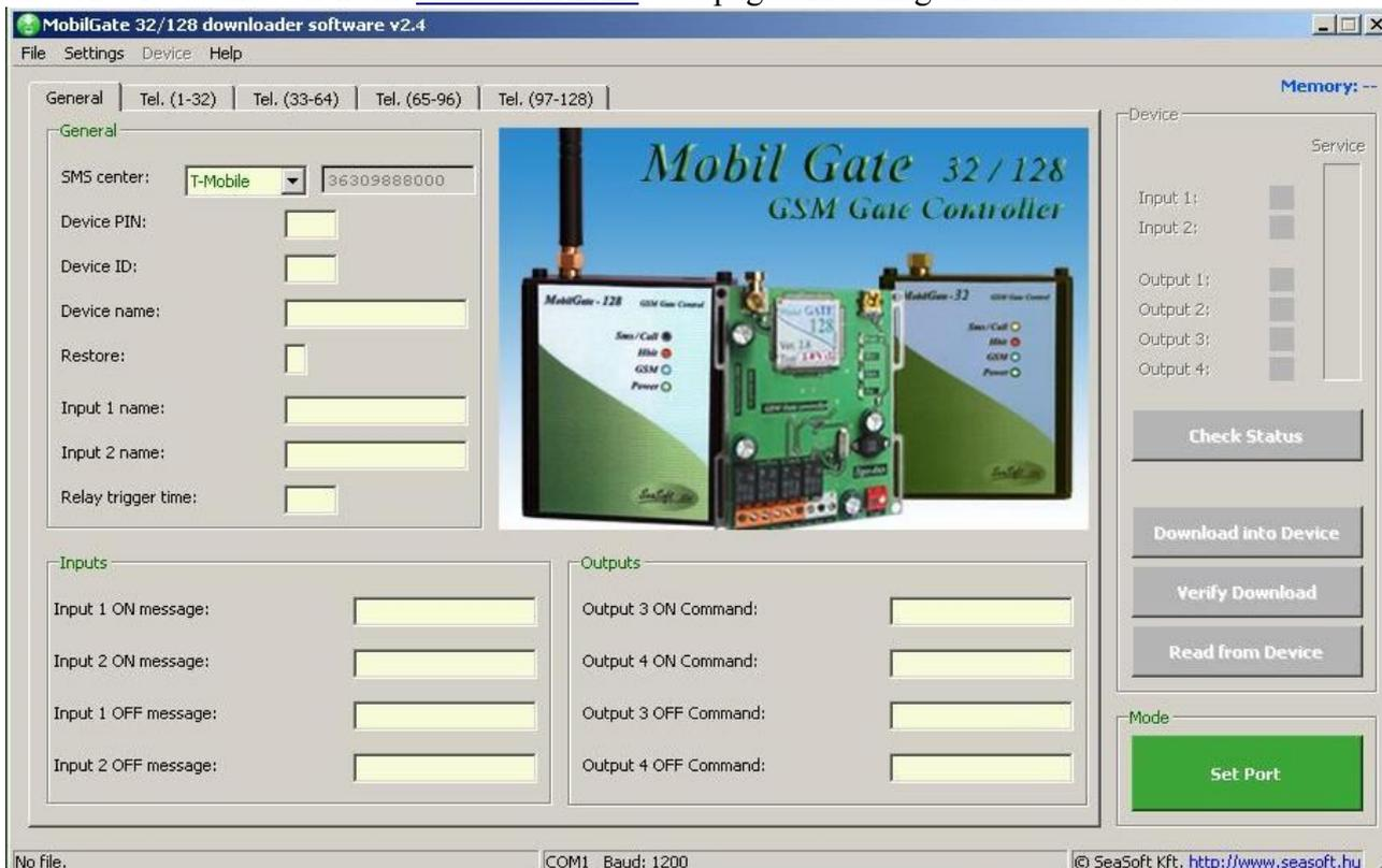
required for Windows XP or any newer operation system to recognize it. During module driver installation, serial port configuration is the next step. It starts by clicking on the **Set Port** button.
