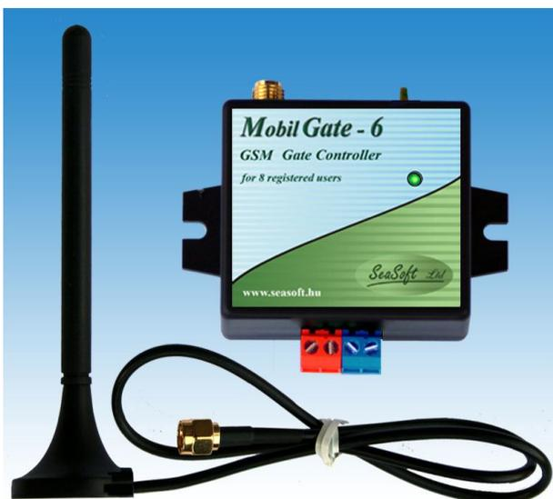
The DC power supply of the **MobilGate-6** device should be connected polarity-wise: the **10-30Vdc** voltage should be connected to the right pin of the red serial connector, and the ground should be connected to the left pin. Should the power supply connected the other way, the device will not be damaged, but will not work either.
