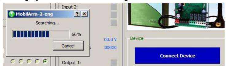
operating system settings should be modified in that particular order as described in the appendix. The software can configure all members of the MobilSwitch family. After connecting the device, launching the software and pressing the “Connect Device” button, the software will automatically search and recognize the
